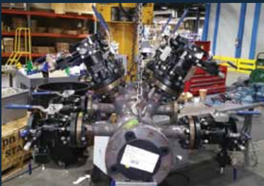
2" PBM TIV on 4 inch ABB Wedge Meter Heavy Crude Line in a Coker Unit
