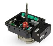
Modular switches with bifurcated reed switches designed specifically for use in low power and high DI card capacitance discrete position feedback applications.
