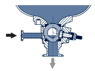
This means on valves mounted vertically like IMI PBM's Angle Stem Flush Tank valve, the valve seals on the <u>upstream</u> seat, thus allowing the body to be purged and drained without process interruption.
