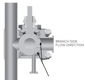
Holes will allow branch side to flow (clean steam/CIP) into valve body and drain through purge port maintaining isolation from run side.
