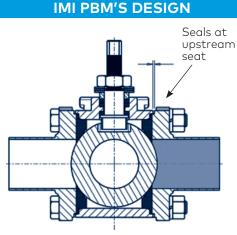
Valve body bolts compress valve seats against the ball, providing bidirectional sealing at the upstream seat. To compensate for seat wear, body bolts can be slightly tightened to re-compress seats against ball.
