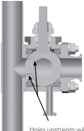
Holes upstream will allow run side to drain.
