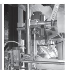
This design offers IMI PBM the ability to provide an ultra-sanitary process isolation valve which seals on both upstream and downstream seats resulting in significant savings compared to traditional methods of using a combination diaphragm valve coupled with a ball valve.
