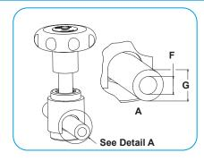
F - Hose ID use for sizing body of valve G - Hose OD use for sizing of safety cover
