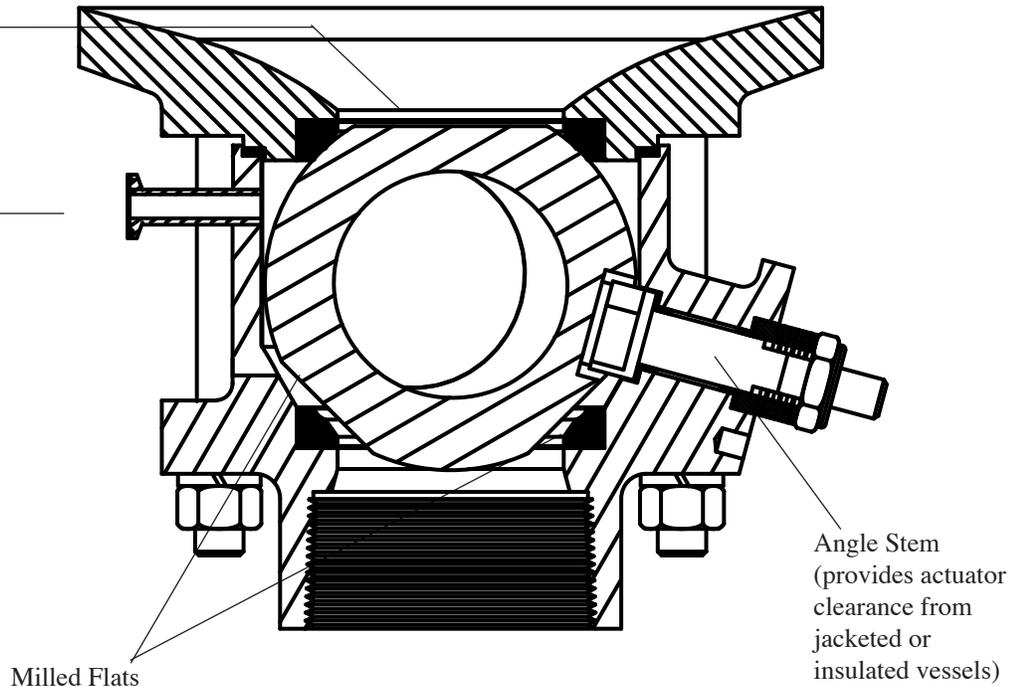
This illustration shows how a single Purge Port and two Milled Flats on the bottom of the ball would work together to flush and drain trapped materials. The valve could also be designed with one inlet and one outlet Purge Port, without Milled Flats, to facilitate the cleaning
