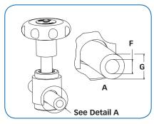
F - Hose ID use for sizing body of valve G - Hose OD use for sizing of safety cover
