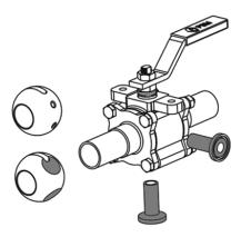
PBM valves seal on the upstream seat unlike conventional floating ball valves.
