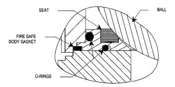
The API-607 qualified valves feature a backup metal seat against which the ball seals if the normal polytetrafluoroethylene seats melt under fire conditions. This metal seal allows only limited leakage under fire conditions.
