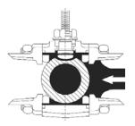
Line pressure pushes ball downstream in ball-closed position, providing seal at downstream seat. Body cavity contains media and pressure. Body cannot be drained or purged during process.
