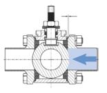
Valve body bolts force valve seats to ball, providing seal at upstream seat. Body cavity can be drained or purged during process.
