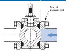
Valve body bolts compress valve seats against ball, providing bidirectional sealing at the upstream seat. To compensate for seat wear, body bolts can be slightly tightened to re-compress seats against ball.
