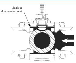
Line pressure pushes ball downstream in the ball-closed position, providing sealing at the downstream seat. There is no adjustment to compensate for seat wear.
