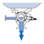
This means on valves mounted vertically, like the pictured PBM angle stem flush tank valve, the valve seats on the upstream seat, thus allowing the body to be purged and drained without process interruption.
